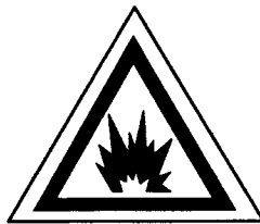
WARNING: EXPLOSIVE ATMOSPHERE
