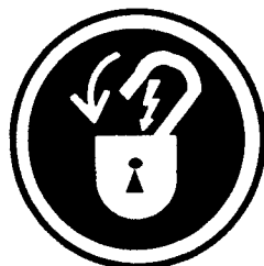
ELECTRICAL LOCKOUT REQUIRED
