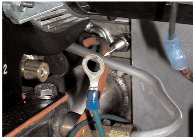
11. Remove ground from ignitor.
