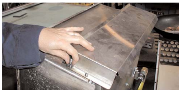
17. Install back guard (washers and acorn nuts).
