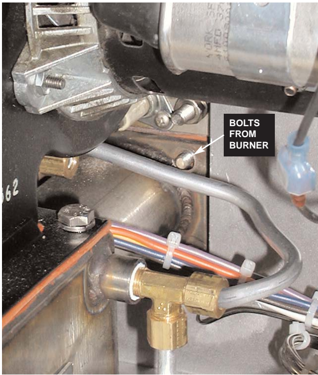
12. Remove four bolts mixing chamber/burner.
