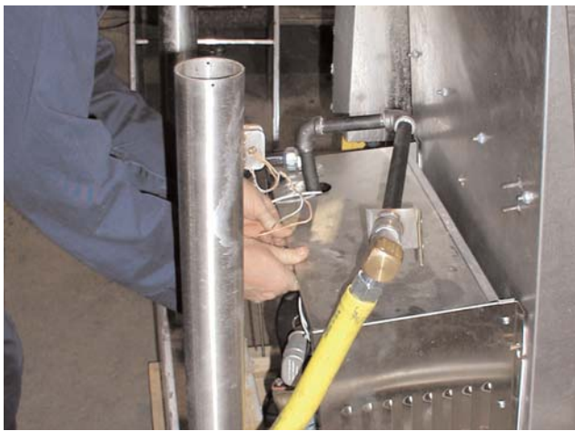
12. Remove four bolts mixing chamber/burner.
