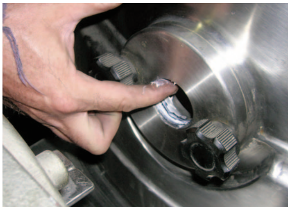
7. Grease seal with food grade grease.
