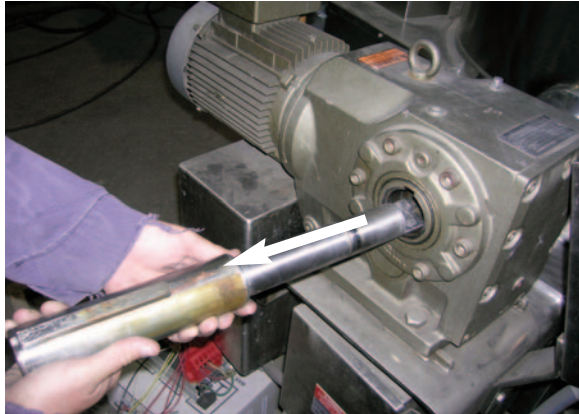
5. Gently hammer out shaft and remove.
