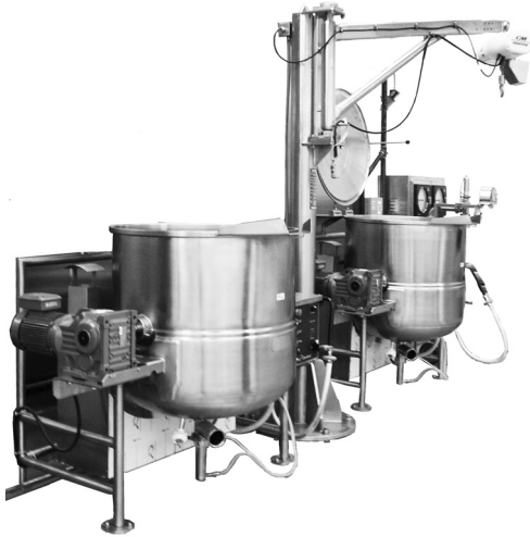
JIB Crane supporting two kettles
