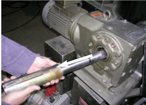
5. Gently hammer out shaft and remove.
