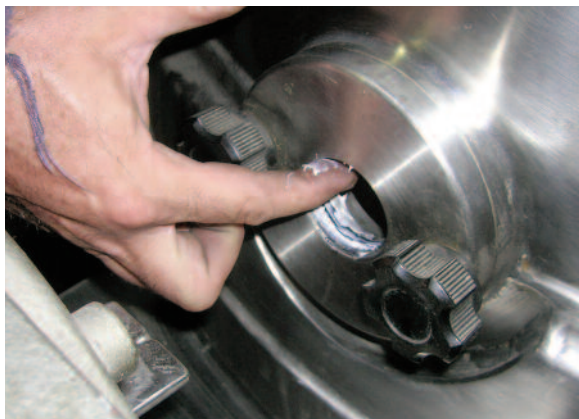
7. Grease seal with food grade grease.
