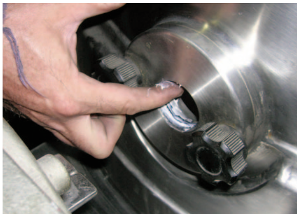
7. Grease seal with food grade grease.
