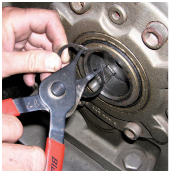
4. Remove shaft retaining ring.
