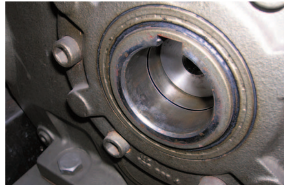
9. Push new shaft past retaining ring groove and install retaining ring.
