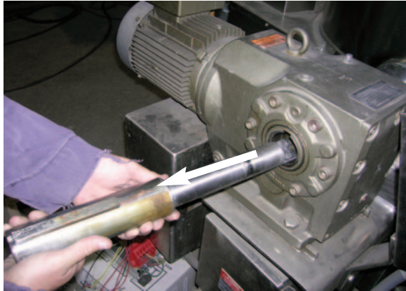
5. Gently hammer out shaft and remove.
