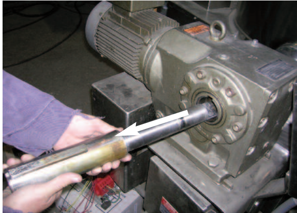
5. Gently hammer out shaft and remove.
