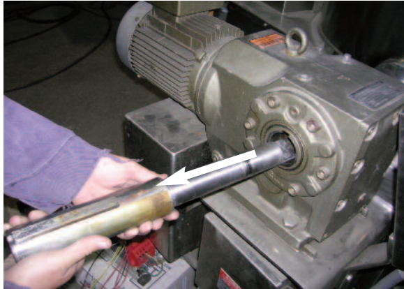
5. Gently hammer out shaft and remove.
