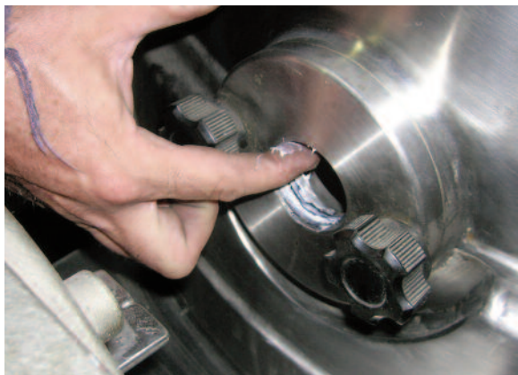
7. Grease seal with food grade grease.
