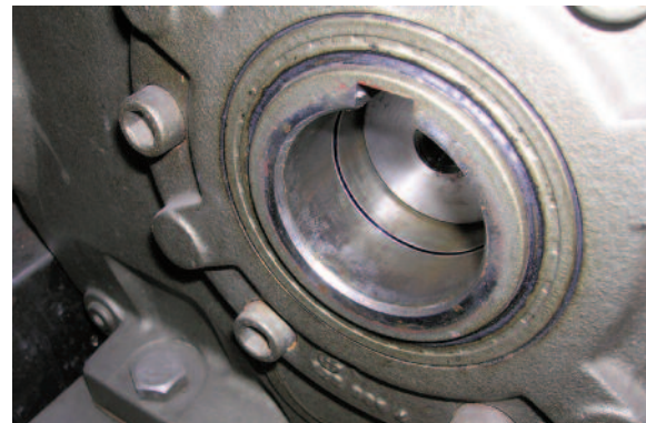
9. Push new shaft past retaining ring groove and install retaining ring.
