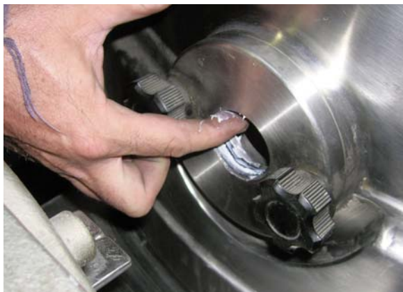
7. Grease seal with food grade grease.
