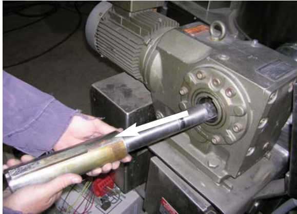
5. Gently hammer out shaft and remove.
