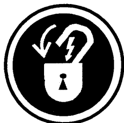
ELECTRICAL LOCKOUT REQUIRED
