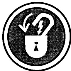
ELECTRICAL LOCKOUT REQUIRED
