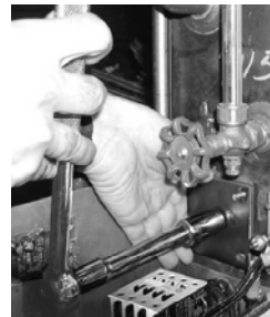
STEP 8 REMOVE #6-32 SCREW FROM CLAMP BAR AND TIGHTEN NUT (25-40 IN.-LBS.) WHILE POSITIONING PLATE OVER HEATER MOUNTING STUD BASES.
