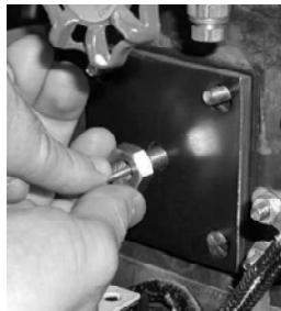
STEP 7 THREAD NUT ONTO CLAMP BAR STUD WHILE HOLDING #6-32 SCREW.
