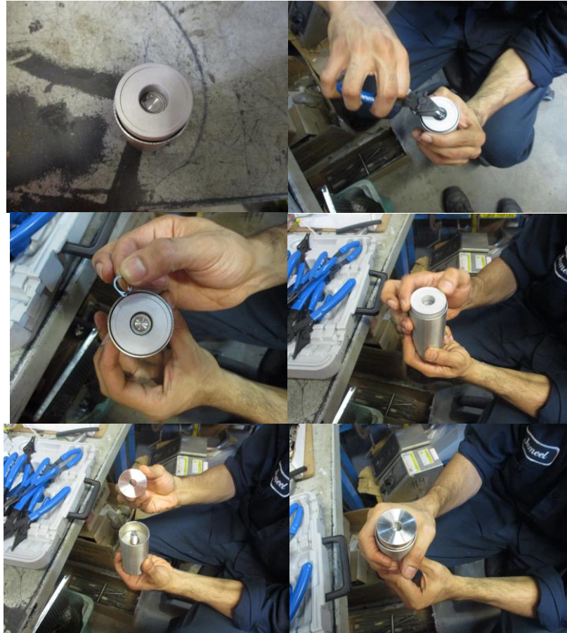
Figure 3 SteamChef™ 6 Re-Placement with new Foot Adapter
