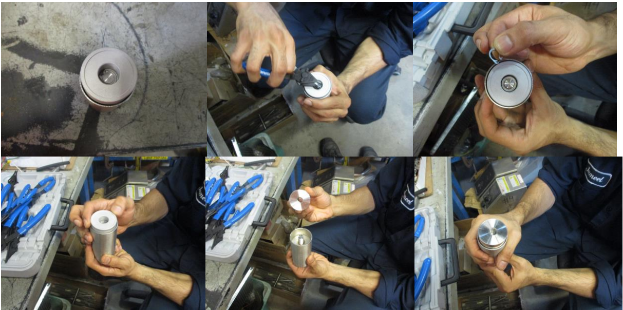
Figure 8 SteamChef™ 6 Re-Placement with new Foot Adapter
