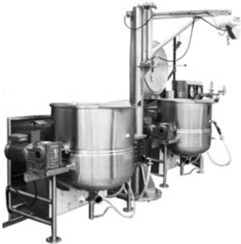
JIB Crane supporting two kettles
