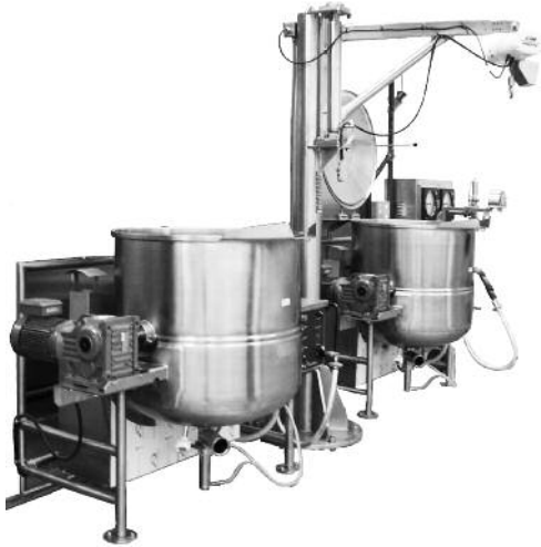
JIB Crane supporting two kettles
