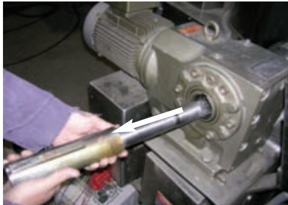
5. Gently hammer out shaft and remove.
