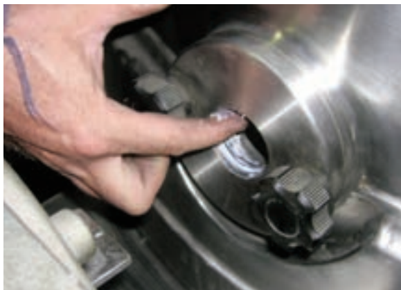
7. Grease seal with food grade grease.
