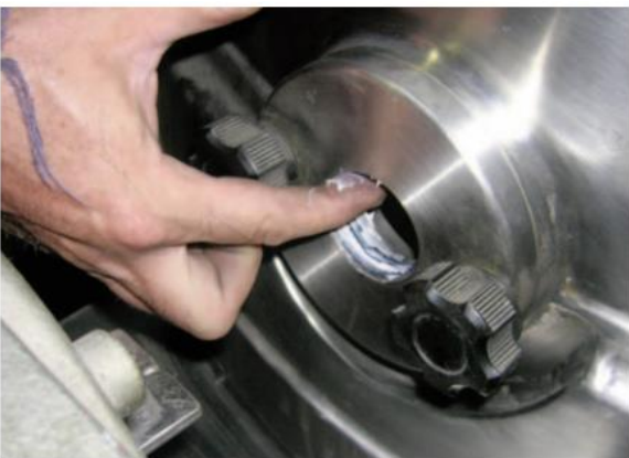
7. Grease seal with food grade grease
