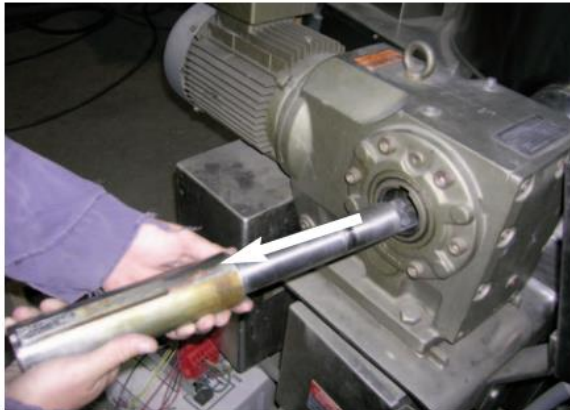
5. Gently hammer out shaft and remove.
