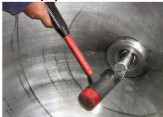
10. Tap shaft to sit up against retaining ring.
