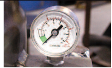
Pressure Gauge in Vacuum.
