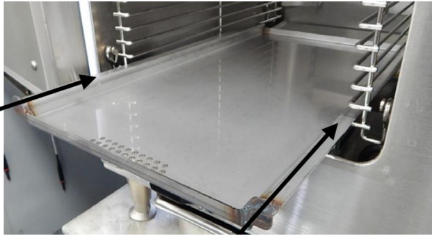
Figure 3-9 Bypass Shield Installation
