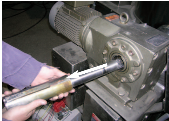
5. Gently hammer out shaft and remove.
