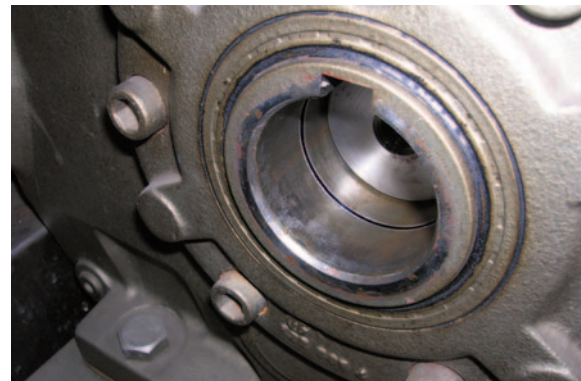
9. Push new shaft past retraining ring groove and install retaining ring.
