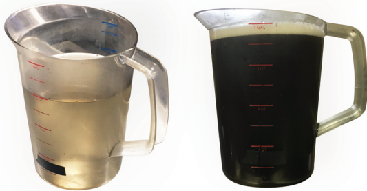
Steam generating water from SteamChef with KleanShield (left) and typical connectionless steam water (right) after 3 loads of potatoes.
