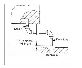
Figure 1. Drain Connections
