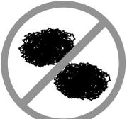
Steel wool should never be used for cleaning the stainless steel.
