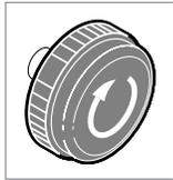
7. When cooking is complete, close the steam control valve by turning the knob clockwise.
