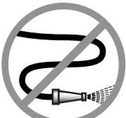
Unit should never be cleaned with a high pressure spray hose.
