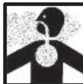
Unit exhaust contains carbon monoxide. Operate only under a properly functioning hood with adequate makeup air.
