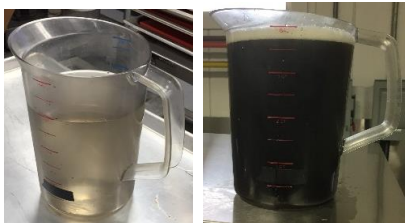
Steam generating water from SteamChef with KleanShield (left) and typical connectionless steam water (right) after 3 pans of potatoes.
